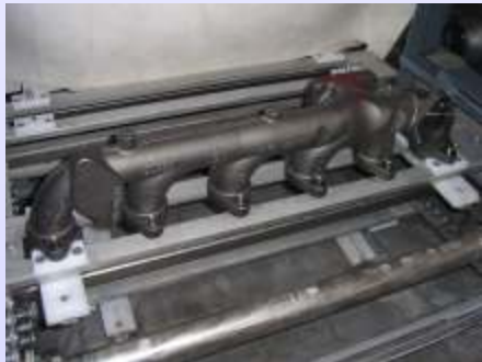
CASTING LOADED IN FIXTURE
